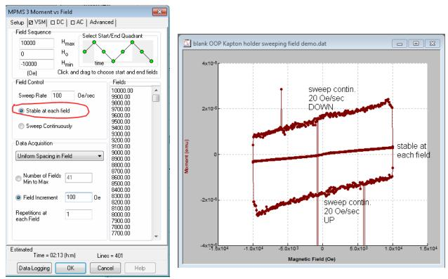
Graph shows the impact of sweeping the field on the M(H) loop of a blank holder with Kapton tape: ~3e-5 emu vertical shift in DOWN vs. UP sweeping data, and noise level is much higher.
