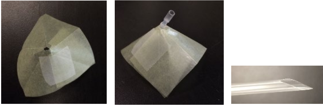
Figure 7: (LEFT) tape the overlapped cut edges; (MIDDLE) a capsule should sit in the hole and not fall; (RIGHT) example of cut straw for spatula. Obtain a tare measurement of capsule + paper using a 0.1mg (or better) sensitivity balance.
