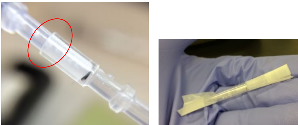
Figure 9: (LEFT) press the two capsules together tightly and wipe up ALL excess grease/powder (red area); (RIGHT) for transporting, put in a clean straw section and tape ends.
