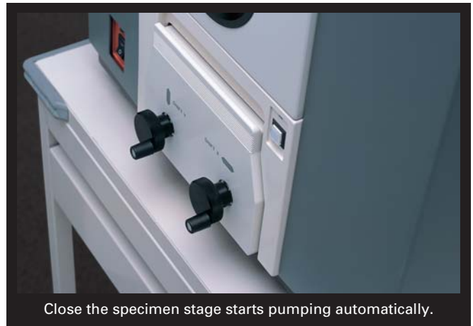
Maximum 70mm diameter \times 50mm height specimen.
