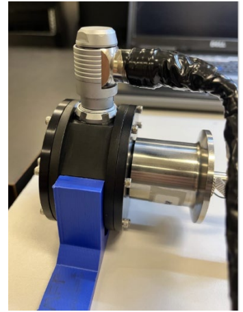
Figure 4: Fischer connector fully seated.
