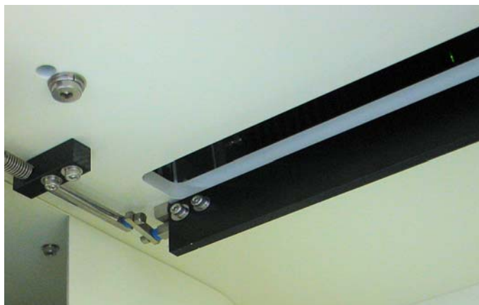
Below the trap door is defeated with a metal scale between the frame and the plunger.
