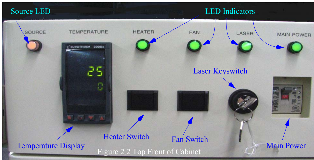
Source Power LED, Temperature Display, Heater Switch, Fan Switch, Laser Keyswitch, and the Main On/Off Switch are located along the top front of the cabinet (Figure 2.2)
