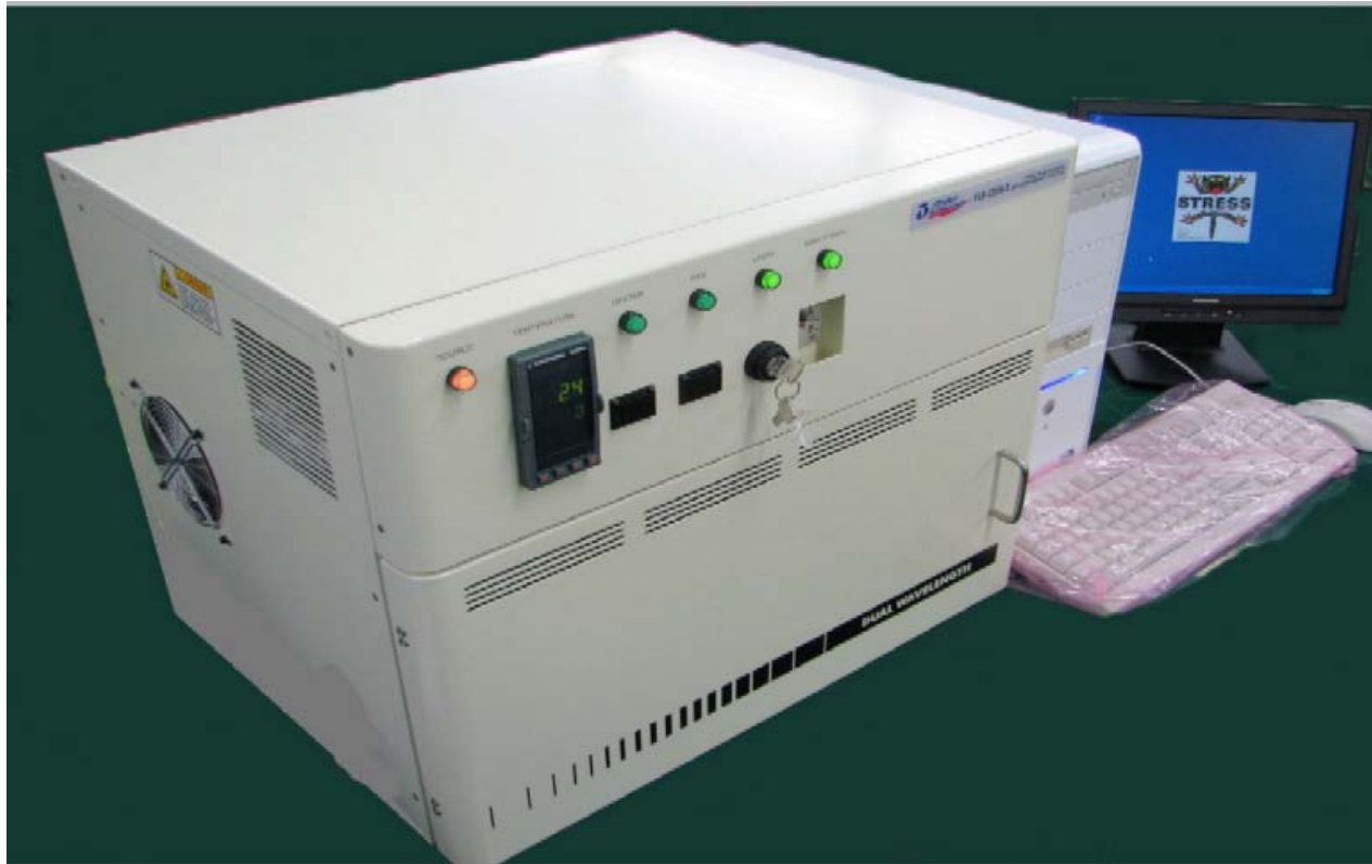
Source Power LED, Temperature Display, Heater Switch, Fan Switch, Laser Keyswitch, and the Main On/Off Switch are located along the top front of the cabinet (Figure 2.2)
