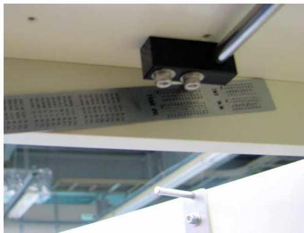
Below the trap door is defeated with a metal scale between the frame and the plunger.
