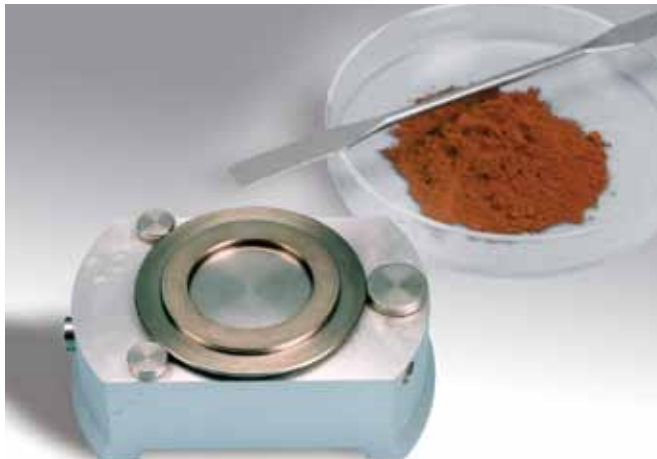
Figure 5. Invert the holder ring and clamp it onto the sample preparation table. Spread the powder into the cavity using a spatula but do not pack or compress.
