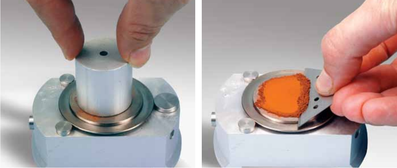
Figure 6. Press powder with the Aluminum block. Remove excess powder with a knife blade or other straight edge.
