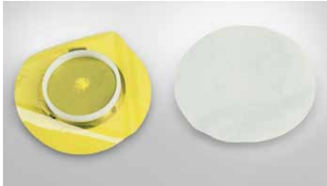
Figure 11. A single sheet of X-ray transparent foil is placed over the zero background plate and the plastic clamping ring seals the foil onto the Sample Holder.
