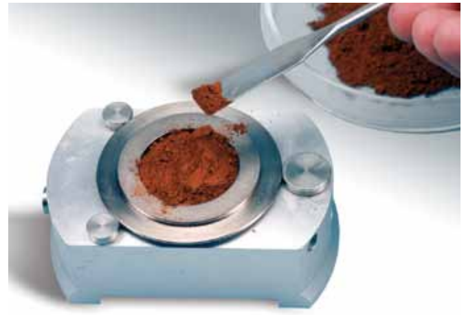
Figure 5. Invert the holder ring and clamp it onto the sample preparation table. Spread the powder into the cavity using a spatula but do not pack or compress.
