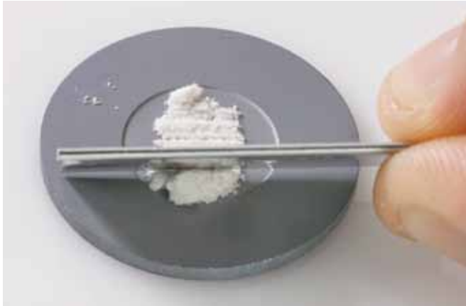
Figure 22. 9430 018 17321 Si 'zero-background' plate. Scrape off excess material with a razor blade, leaving an even uniform surface of material level with the plate surface.
