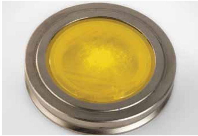
Figure 21. Place the insert into its position in the 9430 018 18401 Sample Holder Ring (a circular spring is not needed to clamp the insert into place).
