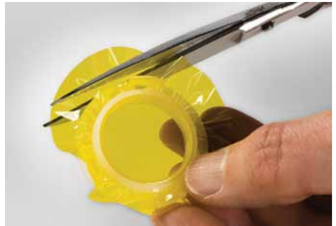
Figure 18. Cut the excess foil extending beyond the circumference of the ring.
