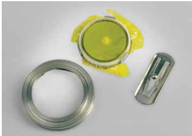
Figure 13. Insert the Sample Holder into the PW1813/40 Sample Holder Ring
