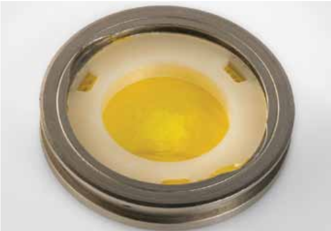
Figure 21. Place the insert into its position in the 9430 018 18401 Sample Holder Ring (a circular spring is not needed to clamp the insert into place).
