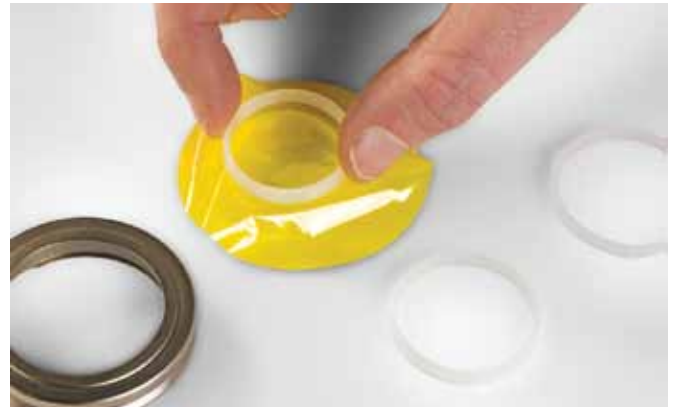
Figure 16. Place the second Kapton foil over the remaining ring with the flat surface and clamp it with the ring that has the three raised bits
