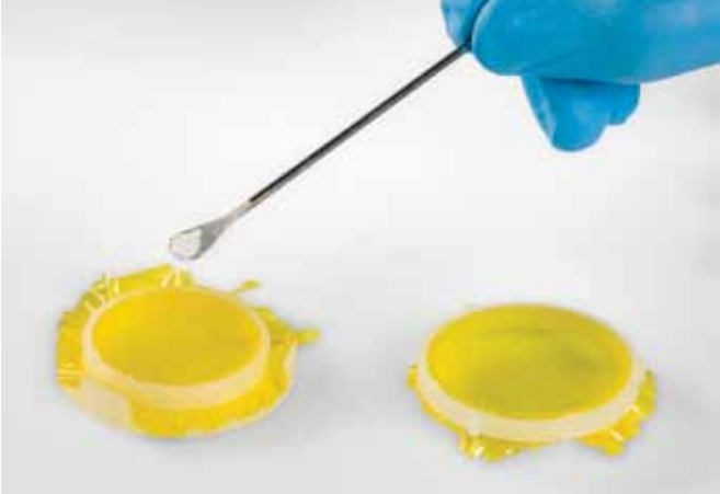
Figure 19. Spread the Sample Material evenly across the center of the foil surface.
