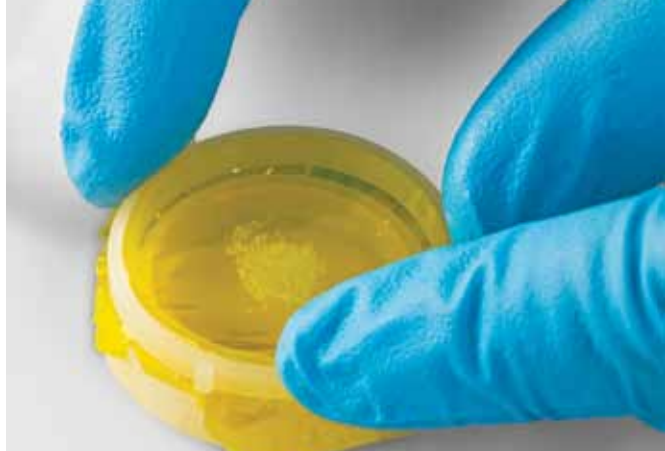
Figure 20. Clamp the Top Part onto the Bottom Part of the Insert
