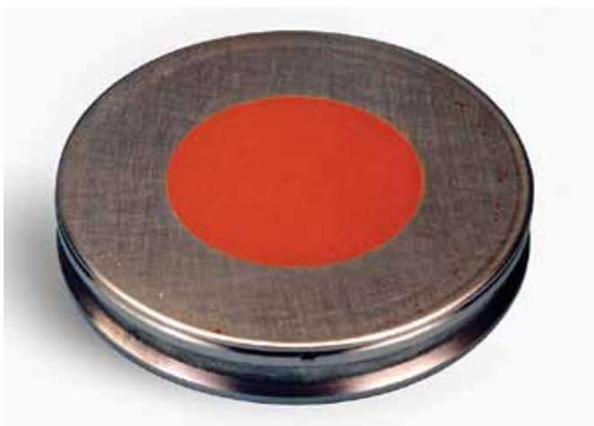
Figure 3. Two-piece round sample holder
