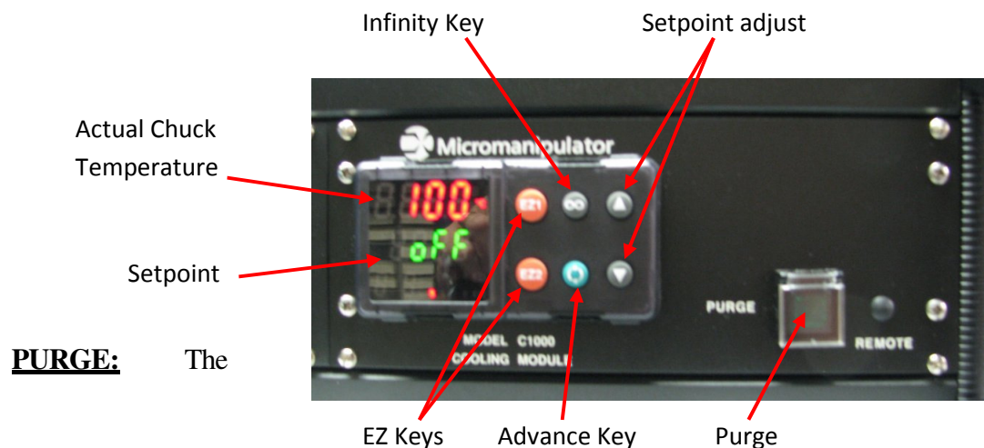
Figure 3.2 Cool Module Controls
