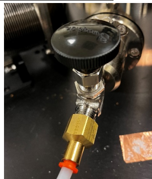
Figure 6. Chamber vent valve
