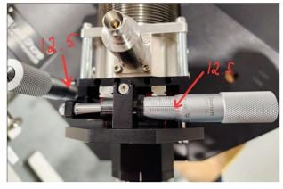
3. Install the locking guide pin, which is boxed in red in the diagram below. You may need to fine-tune both micrometers to ensure that the locking pin is inserted correctly.
