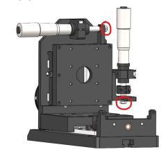
b. To secure the serviced micrometer in place, tighten the micrometer mounting block screw until it is fixed firmly in place. You should not be able to move or twist the micrometer within this block once it is secured.
