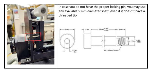
4. **Reference:** Micrometer installation details. Note that the highlighted parts and their installation is identical/repeated for the Y-MICROMETER (but omitted on the drawing to lessen clutter).
