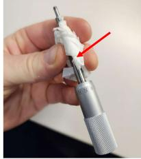
3. Apply a **thin** layer of your preferred general-purpose synthetic lubricant to both ends of the ferrule and apply a thin layer of the same lubricant to the shaft. Reassemble the micrometer by screwing it back together and check for smooth operation throughout the micrometer's range. If your micrometer still feels difficult to turn or has sections that feel hard to move, you may need to replace it.
