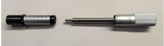
2. Clean both parts of the micrometer using a lab wipe and isopropyl acohol. Wipe down the micrometer shaft and the internal portion of the mating part, especially at both inside ends of the ferrule part.
