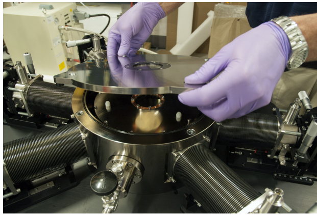
FIGURE 4-3 Probe station vacuum chamber lid removal
