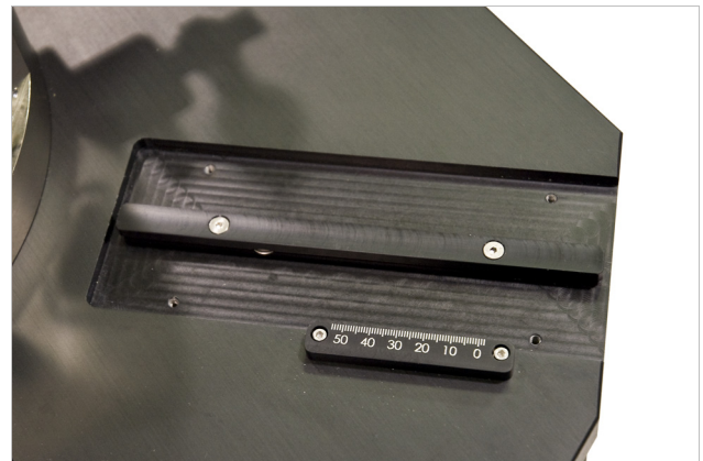
FIGURE 5-2 Left: Remove the screws from the slide insert; Right: Secure the slide insert to the arm stage location
