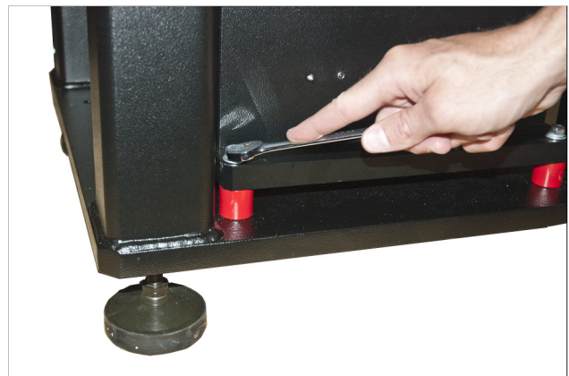
FIGURE 3-11 Left: Vibration isolation pads positioned under the CCR stand feet; Right: Remove the locking bolts and red spacing washers
