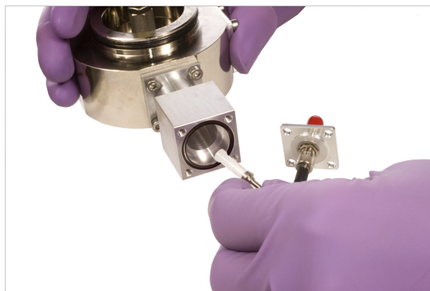
FIGURE 5-21 Insert the optical fiber tip into the feedthrough extension
