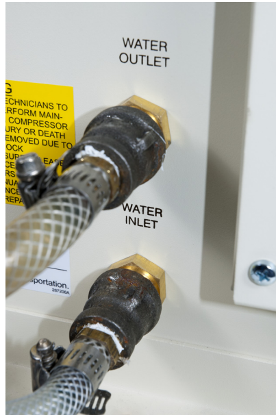
FIGURE 3-10 Water inlet and outlet on the compressor
