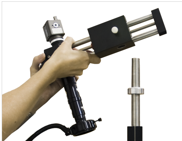
FIGURE 3-22 Installing the horizontal boom onto the vertical post
