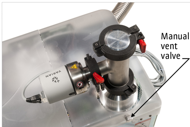
FIGURE 6-3 Turbo vacuum pump NW 40 connection, T, and gauge
