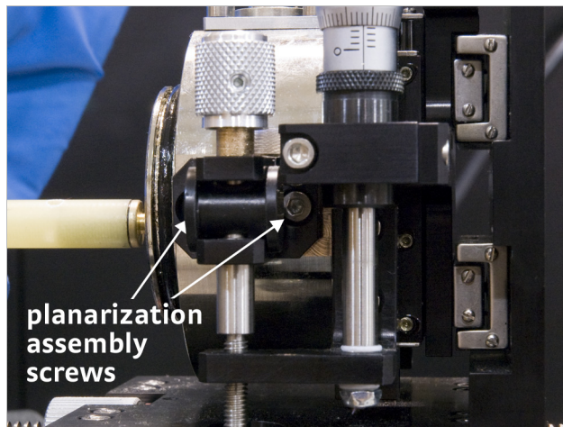
FIGURE 5-10 Left: Loosen the two screws holding the planarization assembly to the probe arm base; Right: Pull out the threaded dowels
