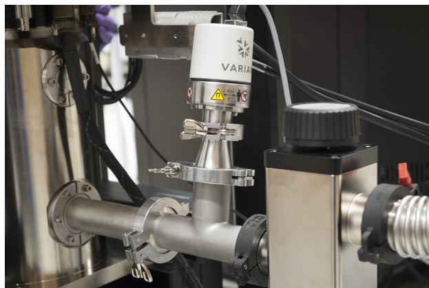
FIGURE 6-4 Vacuum gauge on the CRX-VF vacuum chamber
