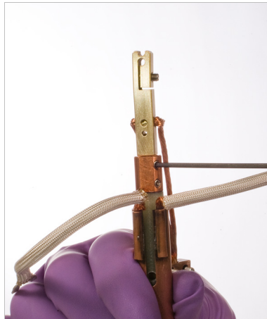
FIGURE 5-19 Secure the probe mount to the probe arm
