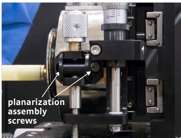
FIGURE 5-12 Left: Securing the planarization assembly to the probe arm base; Right: Taping the cable to the probe arm
