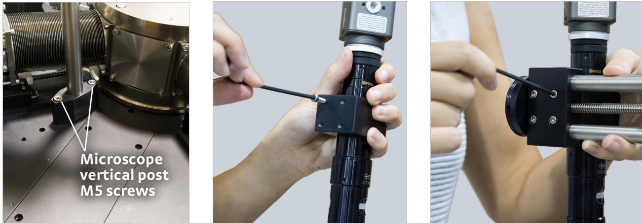
FIGURE 3-21 Left: Installing the microscope vertical post; Middle: Four M3 mounting screws on the vertical post; Right: Attaching the microscope to the horizontal boom
