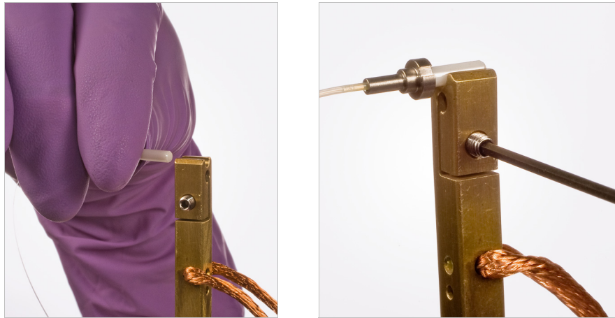
FIGURE 5-22 Left: Inserting the optical fiber tip into the opening in the probe mount; Right: Securing the optical fiber tip by tightening the M3 screw
