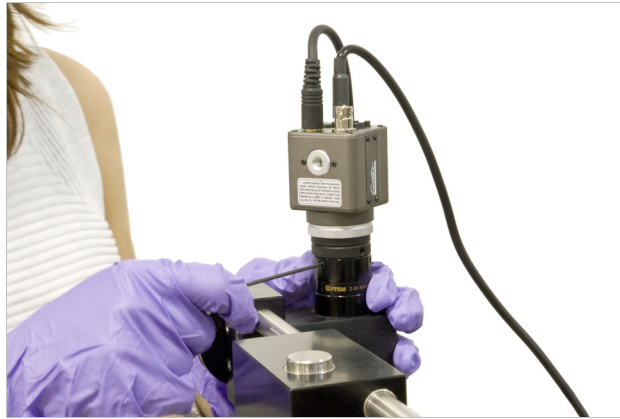
FIGURE 6-7 Loosening the camera rotating joint to adjust the camera image orientation
