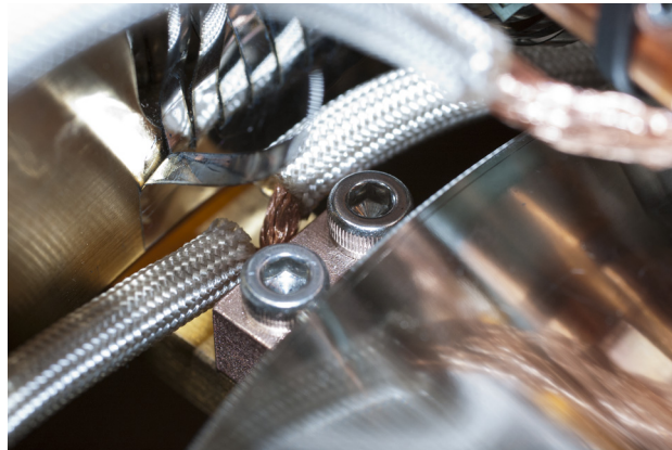
FIGURE 3-33 Braid block mounted to the radiation shield
