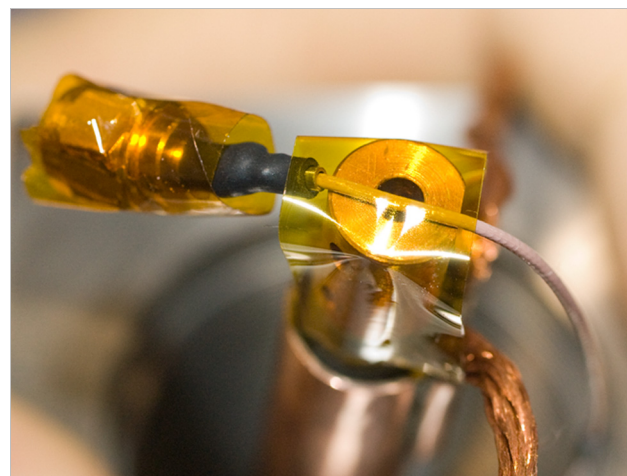
FIGURE 5-12 Left: Securing the planarization assembly to the probe arm base; Right: Taping the cable to the probe arm
